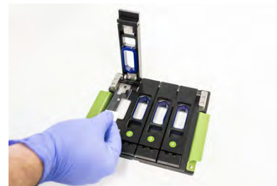
Figure 9: Loading the slide holder
