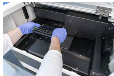
Figure 50: Unloading the slide holder
