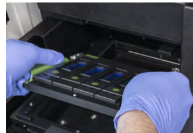
Figure 15: Insert the slide holder onto the stage of the instrument when prompted
