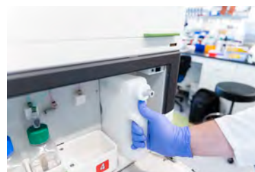
Figure 94: Removing GeoMx DSP waste
