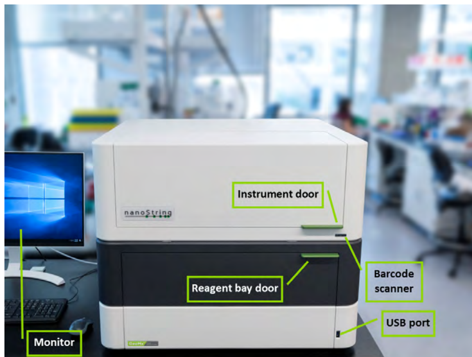
Figure 3: GeoMx DSP instrument exterior diagram
