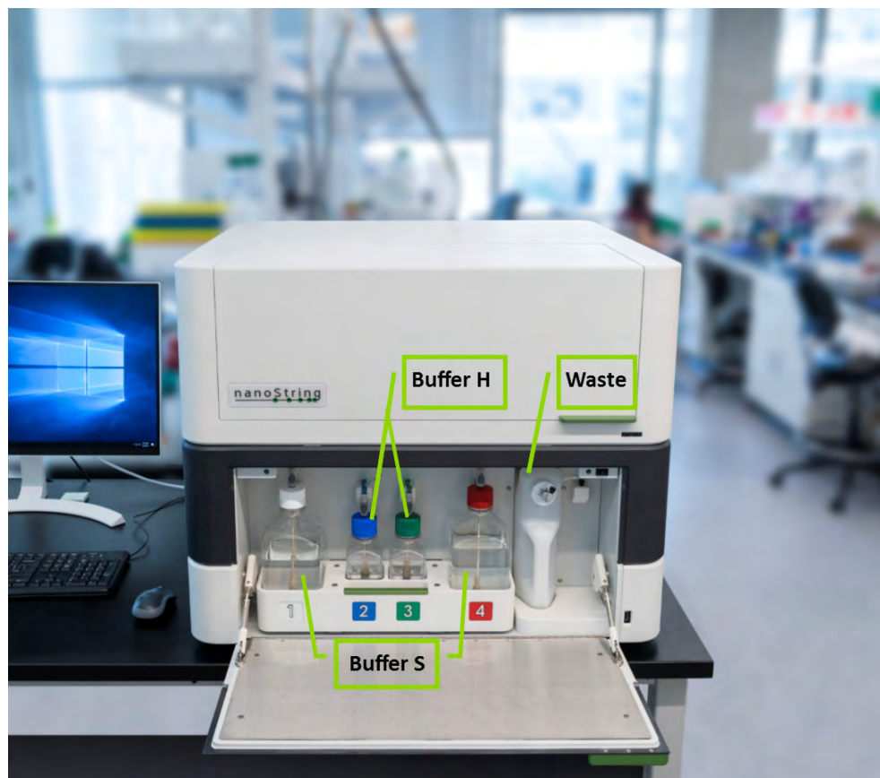
Figure 91: GeoMx DSP instrument reagent bay diagram
