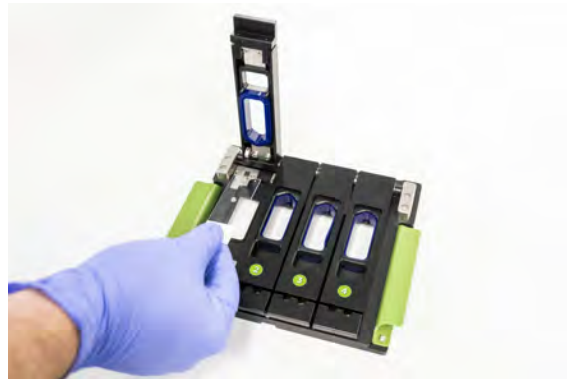
Figure 10: Loading the slide holder
