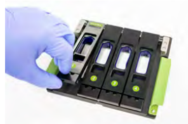
Figure 11: Lowering the slide holder clamps
