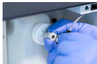
Figure 93: Disconnecting GeoMx DSP waste container
