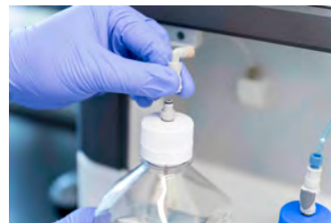
Figure 92: Disconnecting GeoMx reagent bottle
