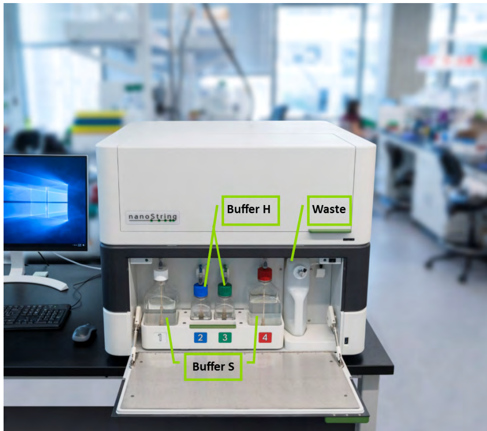
Figure 5: GeoMx DSP instrument reagent bay diagram
