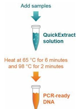
Figure 1. Procedure for using QuickExtract DNA Extraction Solution <sup>[1]</sup>
