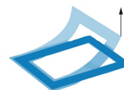
Figure 16: Remove Polyester Frame backing from Incubation Frame
