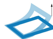
Figure 39: Remove Polyester Frame backing from Incubation Frame
