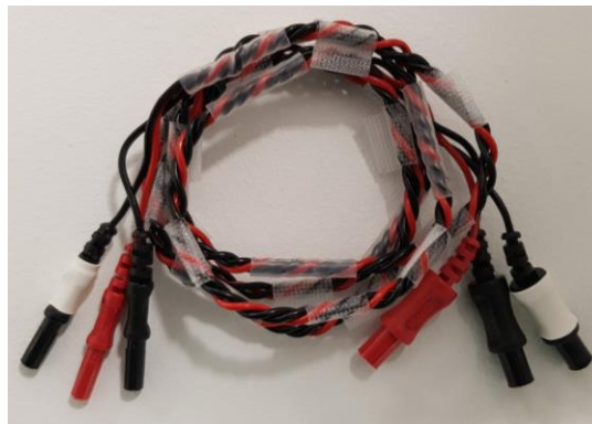
Fig 16: "looping" of excess cable length
