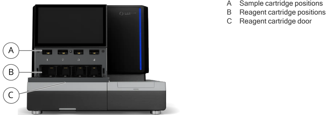
Figure 3 G4X Spatial Sequencer Reagent compartment
