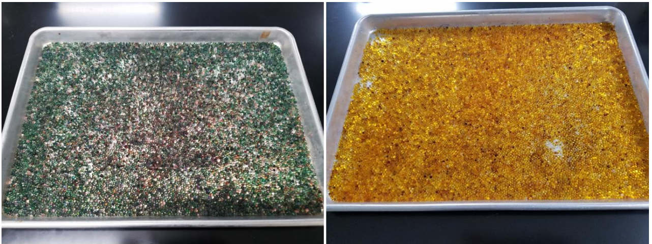
Left panel: Green silica beads before drying. Right panel: silica gel beads after drying.
